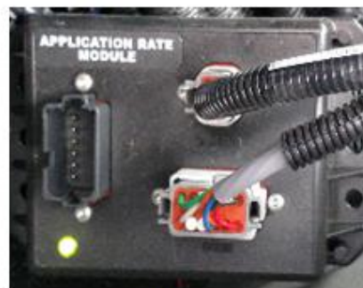
The application rate module communicates with the rate controller via serial interface.
