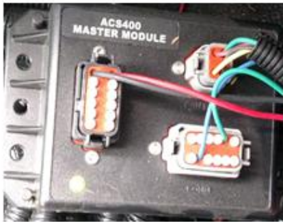
The master module enables connection between the OptRx® sensors and Ag Leader® in-cab monitor.
