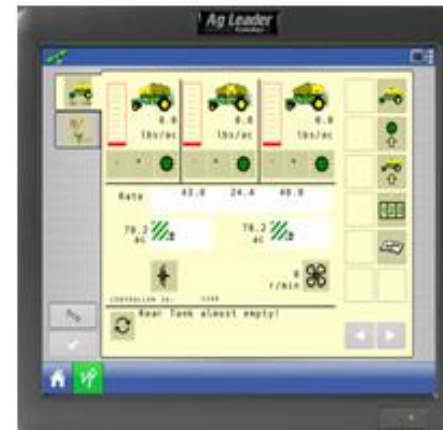
The Ag Leader® monitor receives OptRx® sensor data with ground speed and provides target N ( lb/ac ) to rate controller using a Sufficiency Index algorithm.
