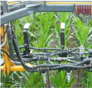
Sensors may be mounted ahead of the applicator boom. Nozzle drops required for liquid N application.
